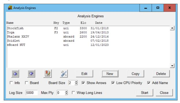
Use the *New* button to add an engine. Give it a name, select the engine file and make sure it is set to use UCI as the protocol:
