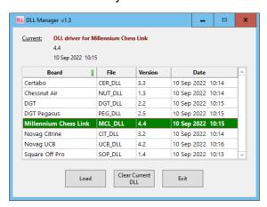
Which boards are listed depends on which drivers you have installed. The top of the screen shows which driver is currently selected (Millennium Chess Link in the above picture). In the list you can choose a different driver and then click *Load* to select it as the current driver. The option to *Clear Current Driver* allows you to revert to the DGT Rabbit Plugin if you have that installed for your DGT board. You do not need to install Rabbit for my drivers.
